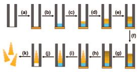
nanowires by gradually changing the composition of a flowing plating solution. The researchers suggest that this versatile method could be adapted to create other nanocale objects with a wide variety of shapes and dimensions.
